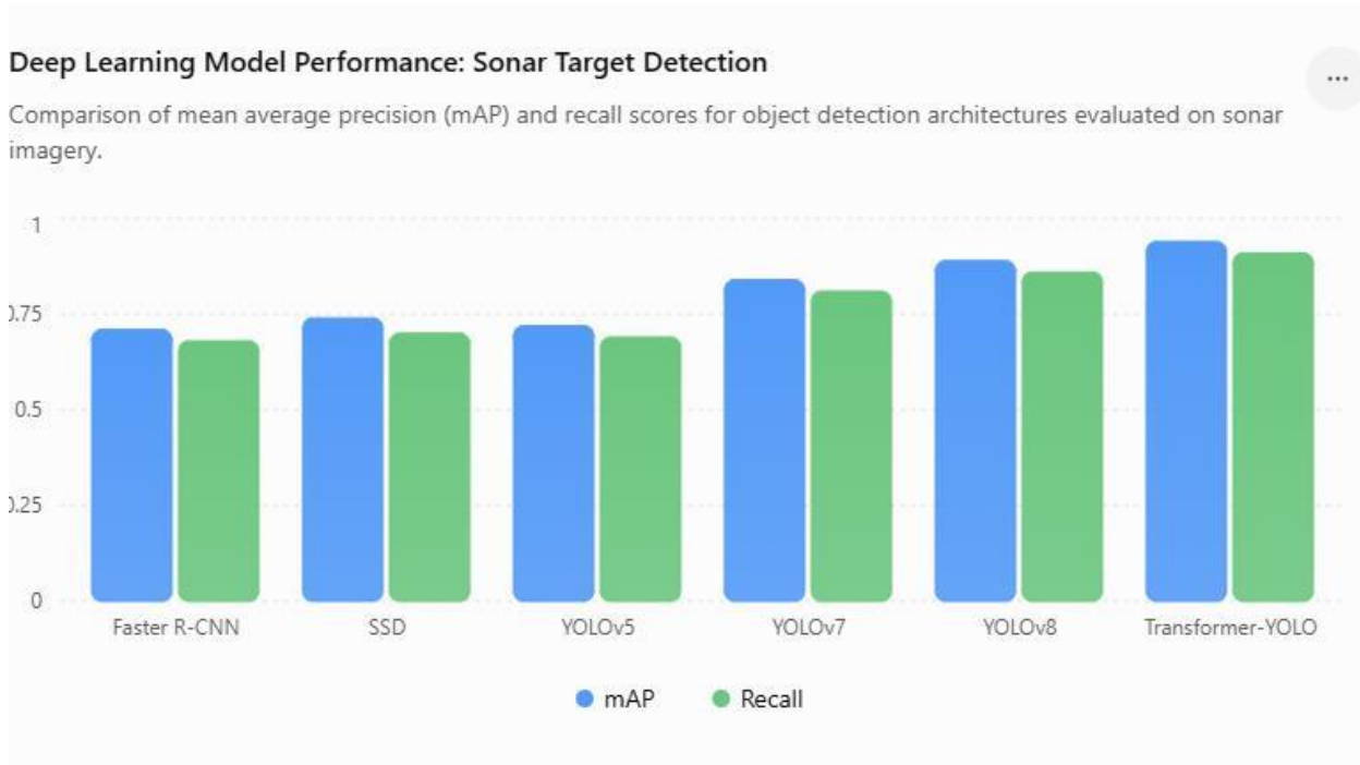
Figure 9. Deep Learning Model Performance: Sonar Target Detection
